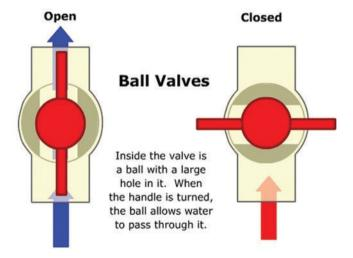
The Graphic to the left illustrates how to turn the Ball Valves to the Closed Position.
