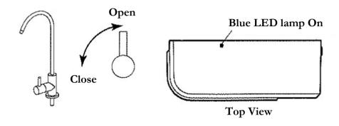
When the faucet valve is closed, the blue LED lamp turns off, the hydrogen generator stops working, and hydrogen generations stops.
